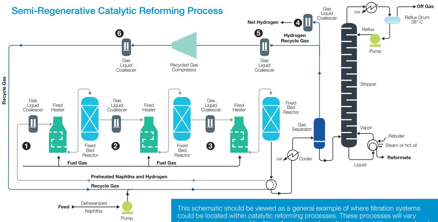
This schematic should be viewed as a general example of where filtration systems could be located within catalytic reforming processes. These processes will vary between companies and facilities. As such, each application should be reviewed and considered individually in order to choose the correct system technology.
