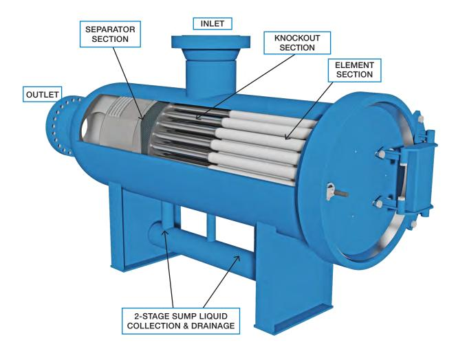
A correctly designed Filter Separator should achieve a maximum turn down of 10:1 and maintain a minimum efficiency of 99.98% of 1 micron and larger and up to 0.3 micron on solids throughout the entire range of operating conditions. Drainage and control of liquids is essential to achieving this efficiency.
